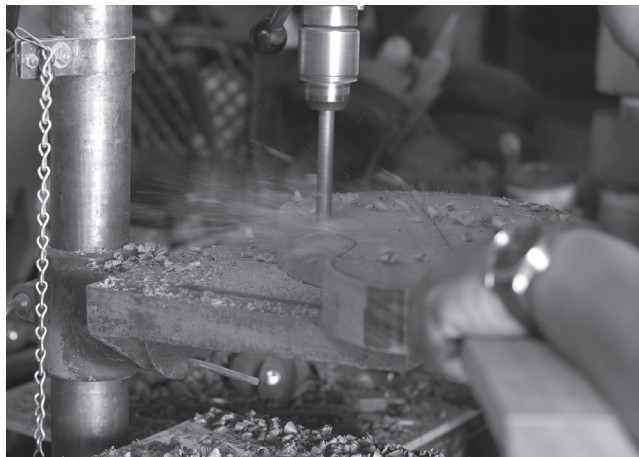
Mena uses a drill press to hollow out his jarana. Jaranas are typically made from one piece of wood, aside from the fret board and top piece of the guitar. The thinner block that Mena is using should give the guitar a shallower tone.
