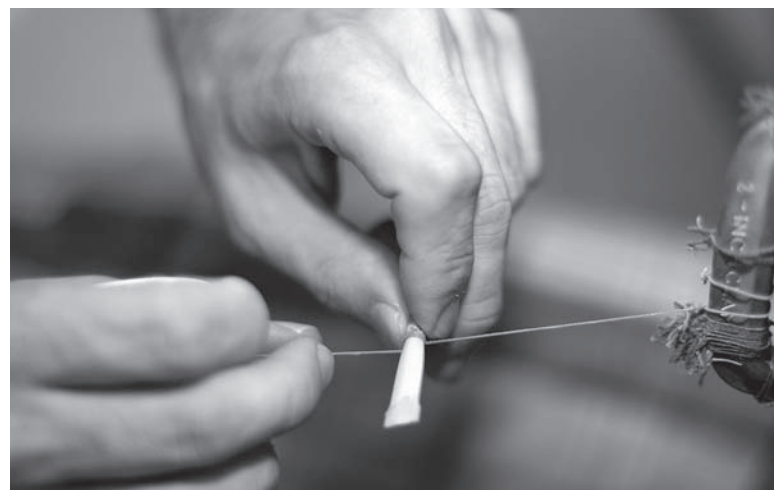
Kennedy ties his reed together with string after he shapes it. The string keeps air from leaking out of the reed as he plays.
